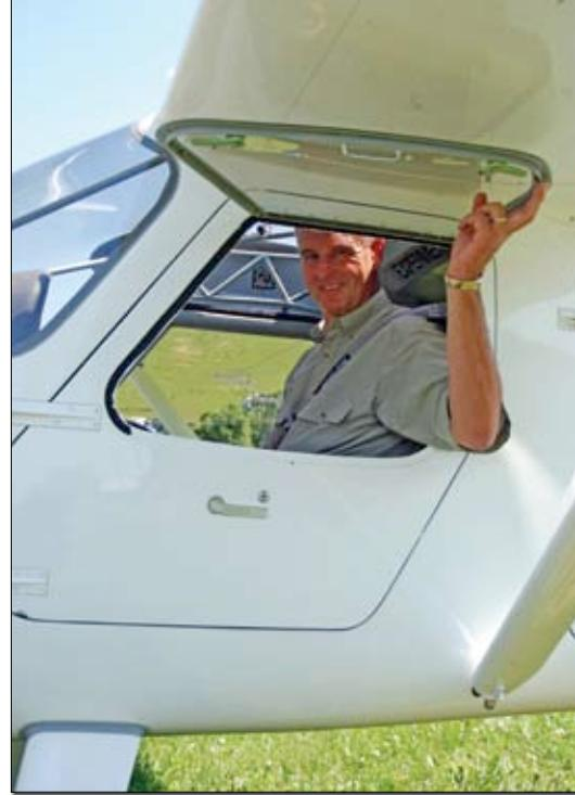
An optional opening window provides a great photo platform but also allows dropping items from a low-flying aircraft.
