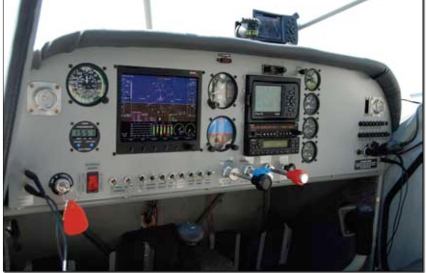
Needham's ship has high-tech equipment—in the form of the Advanced Flight Systems AF-3500 EFIS/engine monitor and TruTrak autopilot—but also backups.
